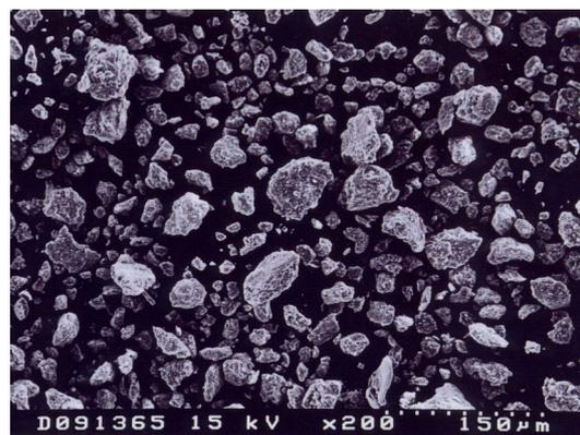
Fig.1 SEM image of cellulose/copper blend prepared by the high speed ball milling for 3 hour
